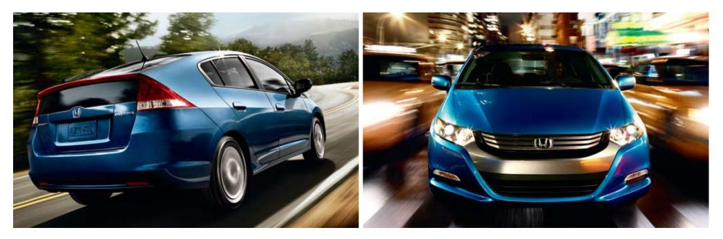
**So what makes an Insight a hybrid?** It's called the Integrated Motor Assist, or IMA<sup>®</sup>. Operating in unison with the already efficient 1.3-litre, i-VTEC<sup>®</sup> 4-cylinder engine, the Insight's advanced fifth-generation IMA powertrain is the ultra-thin compact electric motor that adds power during acceleration and certain cruising situations, and recaptures energy during braking.
