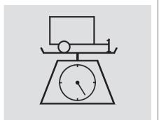
Total Trailer Weight: The maximum allowable weight of the trailer and everything in or on it depends on the number of occupants in your vehicle and the type of trailer being towed (see page 223).
