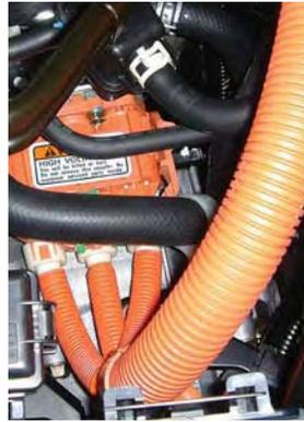
*High-Voltage Cable Connection to Motor*
