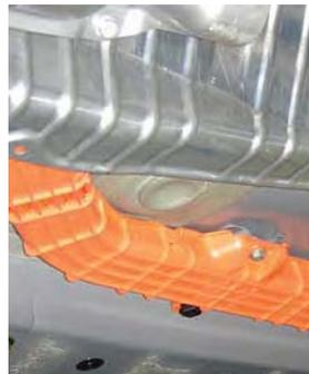
*Electrical shield bolted to undercarriage*
