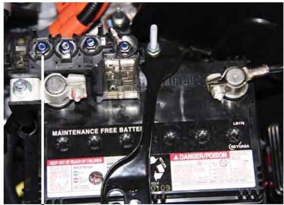
DC to DC Converter Cable Connection
