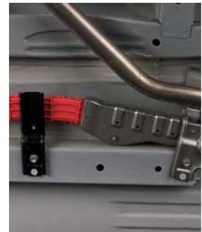
*Thermal shield near hot exhaust*
