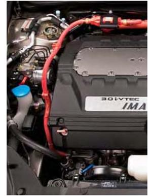
*High-Voltage Cable to Accord AC Compressor*
