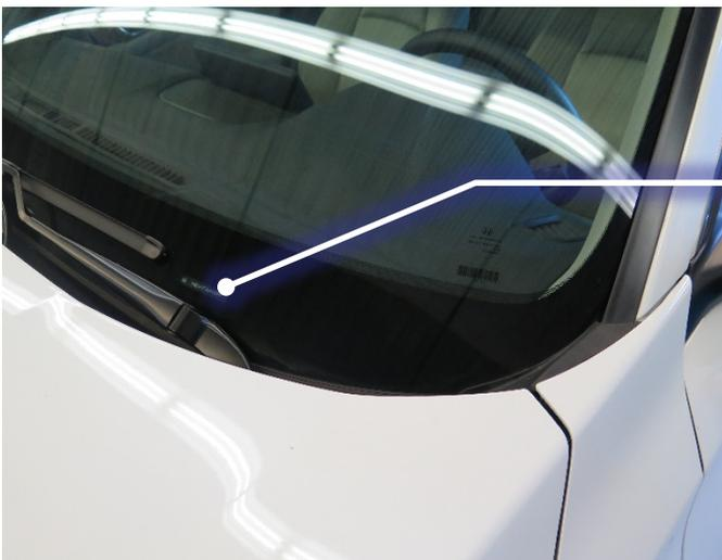
VIN plate located on the lower-right corner of the front windshield.
