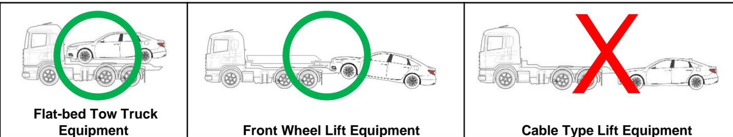
Be aware that when rolling a Honda Accord Hybrid with the front (drive) wheels on the ground, the electric motor can produce electricity and remains a potential source of electric shock even when the high-voltage system is turned off.
