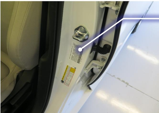
Printed on the VIN label on the driver's door jamb.
