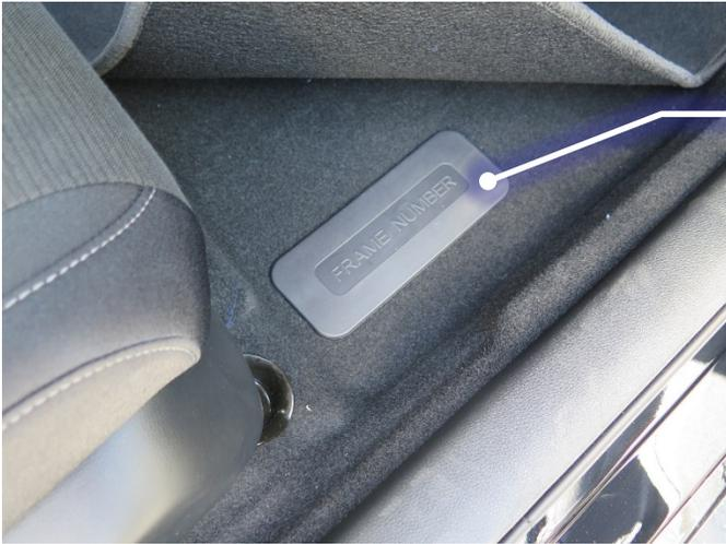
Stamped into the floor panel in front of the passenger seat under a plastic panel marked **FRAME NUMBER**.
