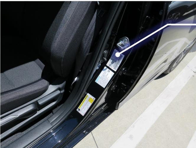
Printed on the VIN label on the driver's door jamb.
