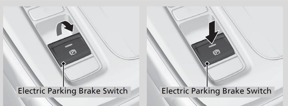
**Applying the Electric Parking Brake**
