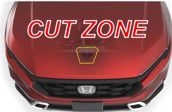
If you need to cut the vehicle body or use Jaws-of-Life equipment to remove occupants, be sure to stay within the cut zone as shown.
