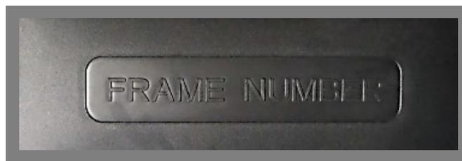
Stamped into the floor panel in front of the passenger seat under a plastic panel marked **FRAME NUMBER**
