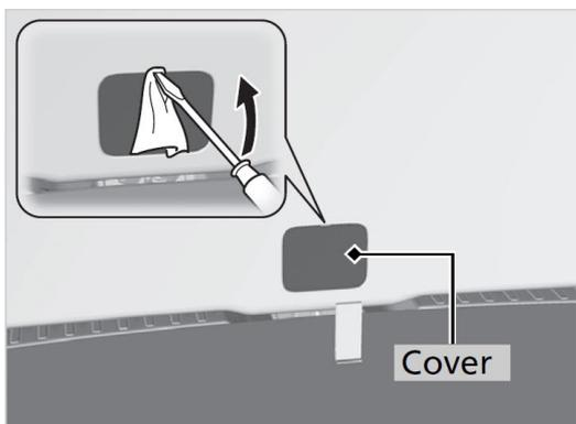
From inside the vehicle, remove the lid on the tailgate panel using a small, flat-tip screwdriver.
