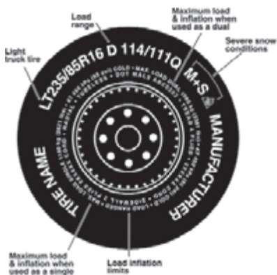
Figure 4: Typical Light Truck Tire Markings
