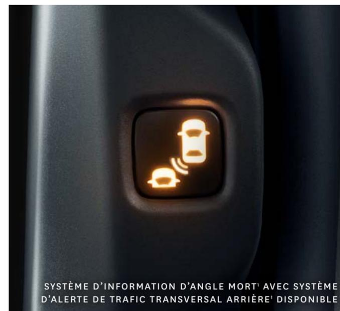
SYSTÈME D'INFORMATION D'ANGLE MORT<sup>1</sup> AVEC SYSTÈME D'ALERTE DE TRAFIC TRANSVERSAL ARRIÈRE<sup>1</sup> DISPONIBLE
