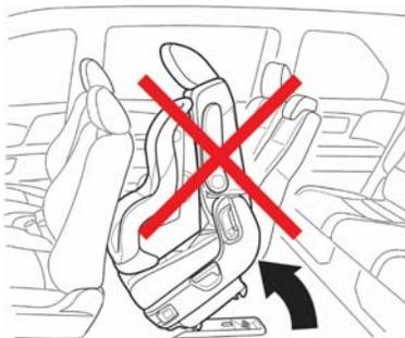
Honda does not recommend using this method to access the third row seats. When the second row outer seat is tipped forward, the seat may slide into the area between the standard and wide positions that prevents the seats from latching. Therefore, using this method of access increases the risk of having an unsecured second row outer seat.
