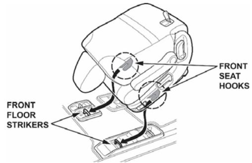
2. Slide the seat into either the standard or wide position.
