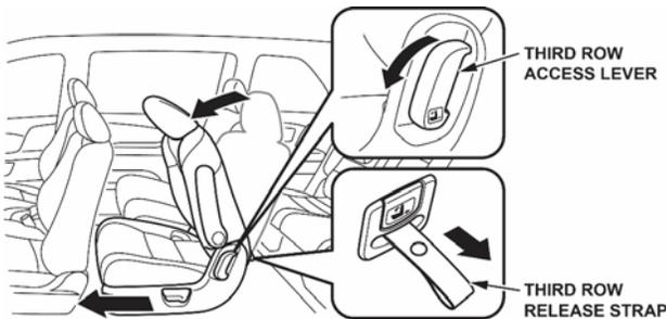
When a child seat is installed in the outer second row seats (typically using the LATCH anchors), the child seat prevents the seat-back from folding forward, which limits access to the third row. Some owners use the seat lock release lever to tip the entire seat forward with the child car seat installed to gain access to the third row.
