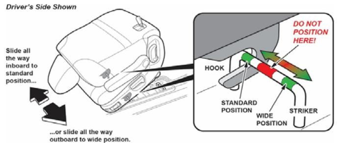
3. Lower the rear of the seat. There is both a rib on the floor and a collar on the rear metal striker. Check that the rear latch and damper are inside or outside of the rib and collar (identified by the green highlight in the illustration):
