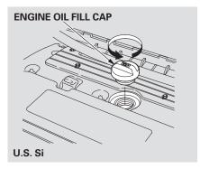
Reinstall the engine oil fill cap, and tighten it securely. Wait a few minutes, and recheck the oil level on the engine oil dipstick. Do not fill above the upper mark; you could damage the engine.
