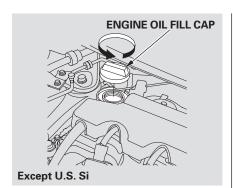
Unscrew and remove the engine oil fill cap on the valve cover. Pour in the oil slowly and carefully so you do not spill any. Clean up any spills immediately. Spilled oil could damage components in the engine compartment.
