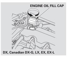
Unscrew and remove the engine oil fill cap on the valve cover. Pour in the oil slowly and carefully so you do not spill any. Clean up any spills immediately. Spilled oil could damage components in the engine compartment.
