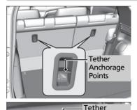
Two tether anchorage points are provided behind the rear outer seating positions and one in the ceiling for the rear center. A child seat that is installed with a seat belt and comes with a tether can use the tether for additional security.
