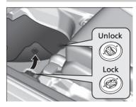
The driver's floor mat hooks over the floor anchors, which keep the mat from sliding forward. To remove a mat for cleaning, turn the anchor knobs to the unlock position. When reinstalling the mat after cleaning, turn the knobs to the lock position.
