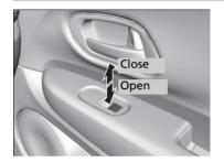
**To open:** Push the switch down lightly, and hold it until the desired position is reached. **To close:** Pull the switch up lightly, and hold it until the desired position is reached.
