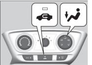
The heater uses heat from the engine coolant to warm the air.
