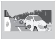
Three lines that appear on the screen can give an idea of how far the vehicles or objects on the screen are from your vehicle, respectively. If an object is near line 1 (in red), it indicates that it is close to your vehicle whereas an object near line 3 farther away.
