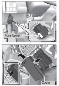
Remove the cover by putting the flat-tip screwdriver into the side slot as shown.
