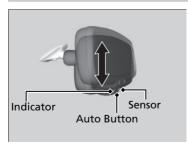
When driving after dark, the automatic dimming rearview mirror reduces the glare from headlights behind you. Press the auto button to turn this function on and off. When activated, the auto indicator comes on. Automatic Dimming Rearview Mirror\*
