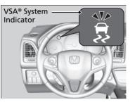
When VSA<sup>®</sup> activates, you may notice that the engine does not respond to the accelerator. You may also notice some noise from the hydraulic system. You will also see the indicator blink. Vehicle Stability Assist (VSA<sup>®</sup>), aka Electronic Stability Control (ESC), System
