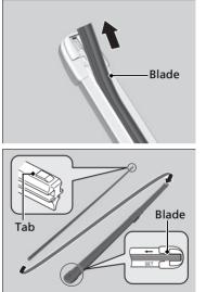
**3.** Slide the wiper blade out from its holder by pulling the tabbed end out.
