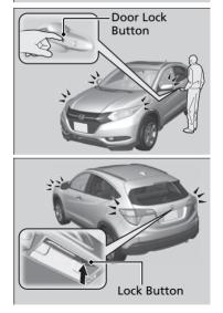
When you carry the smart entry remote, you can lock/unlock the doors and the tailgate. You can lock/unlock the doors and the tailgate within a radius of about 32 inches (80 cm) of the outside door handle. You can open the tailgate within about 32 inches (80 cm) radius from the tailgate release button.
