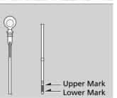
4. Remove the dipstick again, and check the level. It should be between the upper and
