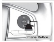
Press the (distance) button to change the ACC with LSF following interval.
