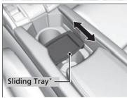
You can put small items in the sliding tray\* located in the console compartment lid. Slide the sliding tray forward or rearward.
