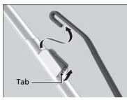
**4.** Press and hold the tab, then slide the blade out from the wiper arm.
