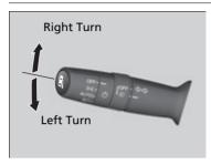
The turn signals can be used when the ignition switch is in ON  $\overline{II}$ <sup>\*1</sup>.
