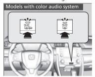
The rear defogger and heated door mirrors automatically switch off after 10-30 minutes depending on the outside temperature. However, if the outside temperature is 32°F (0°C) or below, they do not automatically switch off.
