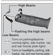
Rotating the light switch turns the lights on and off, regardless of the power mode setting or position of the ignition switch.
