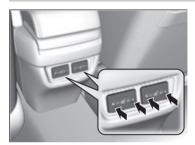
The ignition switch must be in ON  $\boxed{II}^{*1}$  to use the seat heaters. The **HI** setting heats the seats faster than the **LO** setting.
