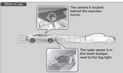
The system starts monitoring the roadway ahead when your vehicle speed is about 3 mph (5 km/h) and there is a vehicle in front of you.
