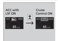
Press and hold the (distance) button for one second. **Cruise Mode Selected** appears on the driver information interface for two seconds, and then the mode switches to Cruise.
