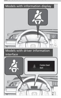
Your vehicle monitors front seat belt use. If the ignition switch is turned to ON II \*1 before the driver's seat belt is fastened, the beeper will sound and the indicator will blink. If the driver does not fasten the belt before the beeper stops, the indicator will remain on.
