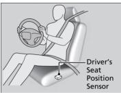
The driver's advanced front airbag system includes a seat position sensor.
