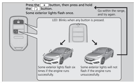
When started remotely, the engine automatically shuts off after 10 minutes of idling and the brake pedal and **ENGINE START/STOP** button have not been pressed simultaneously.
