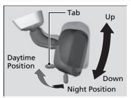
Flip the tab to switch the position.
