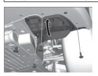
**1.** Remove the clips using a flat-tip screwdriver, remove the bolt, and push up the under cover.
