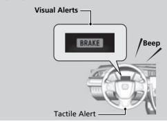
At system's earliest collision alert stage, you can change the distance (**Long/Normal/Short**) between vehicles at which alerts will come on through audio/information screen setting options.
