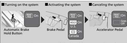
Fasten your seat belt properly, then start the engine. Press the automatic brake hold button.
