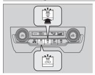
Pressing the (windshield defroster) button automatically switches the system to fresh air mode.
