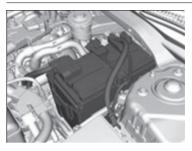
Check the battery terminals for corrosion monthly.
