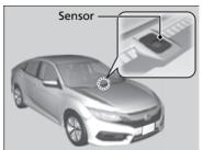
The automatic heating system is equipped with sensors. Do not cover or spill any liquid on them.
