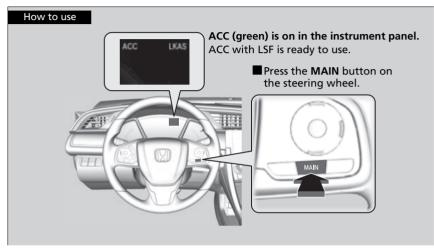
When the **MAIN** button is pressed, both ACC with LSF and the Lane Keeping Assist System (LKAS) are either turned on or off.
