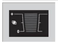
When the turbo charger is activated, this meter shows the boost pressure.
