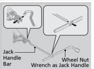
Raise the vehicle, using the jack handle bar and the jack handle, until the tire is off the ground.
