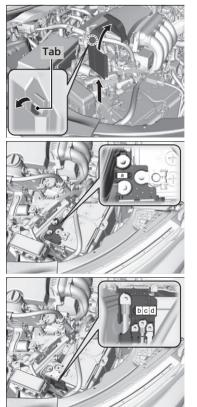
Pull up the cover on the  $\oplus$  terminal, then remove it while pulling out the tab as shown.
