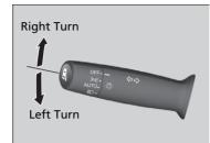
The turn signals can be used when the power mode is in ON.
