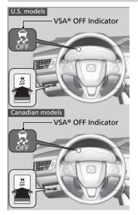
This button is on the driver side control panel. To partially disable VSA<sup>®</sup> functionality/ features, press and hold it until you hear a beep.
