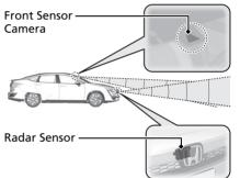
The radar sensor is inside the front grille.
