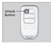
**To open:** Press the unlock button, and then within 10 seconds, press it again and hold it.
