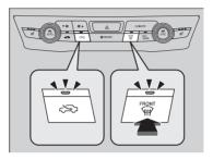
Pressing the result button turns the air conditioning system on and automatically switches the system to fresh air mode.
