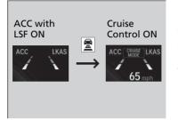
Press and hold the 🖹 (interval) button for one second. **Cruise Mode Selected** appears on the driver information interface for two seconds, and then the mode switches to Cruise.
