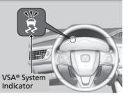
When VSA<sup>®</sup> activates, you may notice that the engine and motor do not respond to the accelerator. You may also notice some noise from the hydraulic system. You will also see the indicator blink. Vehicle Stability Assist (VSA<sup>®</sup>), aka Electronic Stability Control (ESC), System
