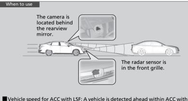
Vehicle speed for ACC with LSF: A vehicle is detected ahead within ACC with LSF range – ACC with LSF operates at speeds up to 90 mph (145 km/h). No vehicle is detected within ACC with LSF range – ACC with LSF operates at the speed of 25 mph (40 km/h) or above.
