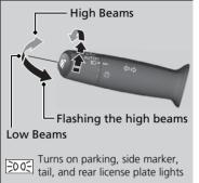
Turns on headlights, parking, side marker, tail, and rear license plate lights Rotating the light switch turns the lights on and off, regardless of the power mode setting.
