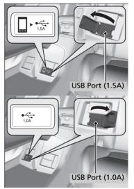
Install the device USB connector or the USB flash drive to the USB port.
