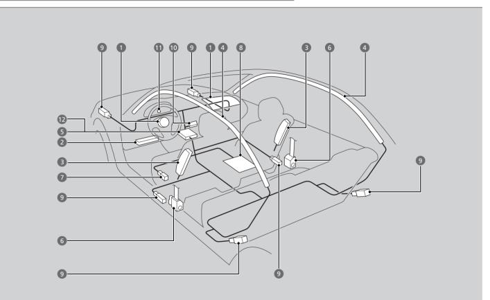
The front, driver's knee, front side, and side curtain airbags are deployed according to the direction and severity of impact. Both side curtain airbags are deployed in a rollover. The airbag system includes:
