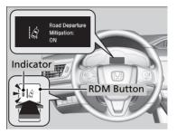
Press the RDM button to turn the system on and off.
