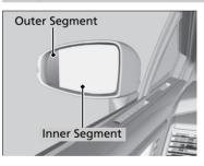
The driver's side door mirror has outer and inner segments.
