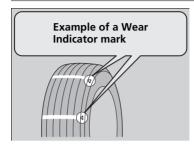
The groove where the wear indicator is located is 1/16 inch (1.6 mm) shallower than elsewhere on the tire. If the tread has worn so that the indicator is exposed, replace the tire. **Worn out tires have poor traction on wet roads.**
