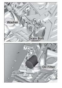
**4.** Remove the drain bolt and washer from the bottom of the engine, and drain the oil into a suitable container.
