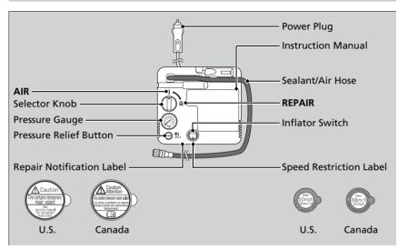
Setting Ready to Temporarily Repair the Flat Tire
