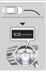
The front camera behind the rearview mirror monitors left and right lane markings (in white or yellow). If your vehicle is getting too close to detected lane markings without a turn signal activated, the system, in addition to a visual alert, applies steering torque and alerts you with rapid vibrations on the steering wheel, to help you remain within the detected lane. Customized Features P. 306
