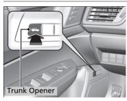
Pressing the trunk opener on the driver's door unlocks and opens the trunk. When You Cannot Open the Trunk P. 564
