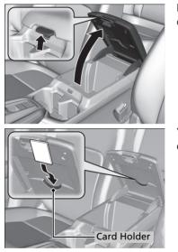
Pull the handle to open the console compartment.
