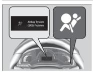
■ When the power mode is set to ON The indicator comes on for a few seconds, then goes off. This tells you the system is working properly. Supplemental Restraint System (SRS) Indicator
