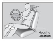
The driver's knee airbag is housed under the steering column.
