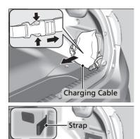
**1.** Remove the charging cable by releasing the belt.
