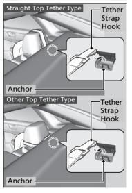
A tether anchorage point is provided behind each rear seating position.
