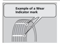
The groove where the wear indicator is located is about 1/16 inch (about 1.6 mm) shallower than elsewhere on the tire. If the tread has worn so that the indicator is exposed, replace the tire.
