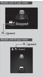
Your vehicle also stops, automatically. The **Stopped** message appears on the gauge. When the vehicle ahead of you starts again, if you press the **RES/+/SET/-** switch up or down, or depress the accelerator pedal, ACC with Low Speed Follow will operate again within the prior set speed.
