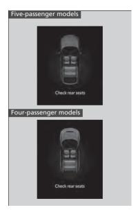
A reminder appears on the driver information interface and an alert will sound when the power mode is set to VEHICLE OFF.
