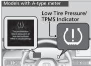
This will cause the low tire pressure/TPMS indicator to come on and a message to appear on the gauge.
