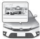
When finished, close the hood and make sure it is firmly locked in place.
