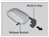
The built-in key can be used to unlock the doors when the keyless remote battery becomes weak and the power door unlock operation is disabled.
