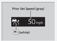
The set speed cannot be set or resumed when ACC has been turned off using the substantial button. Press the button to activate the system, then set the desired speed.
