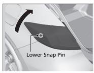
**3.** Grasp underneath the taillight and rotate it upward to release the lower snap pin.
