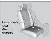
The front passenger's advanced airbag system has weight sensors. The sensors are used for occupant classification to activate or deactivate the front passenger's airbag.
