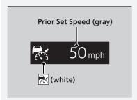
The set speed cannot be set or resumed when ACC with Low Speed Follow has been turned off using the button. Press the button to activate the system, then set the desired speed.
