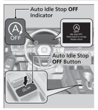
To turn the Auto Idle Stop system off, press this button. The Auto Idle Stop system stops.
