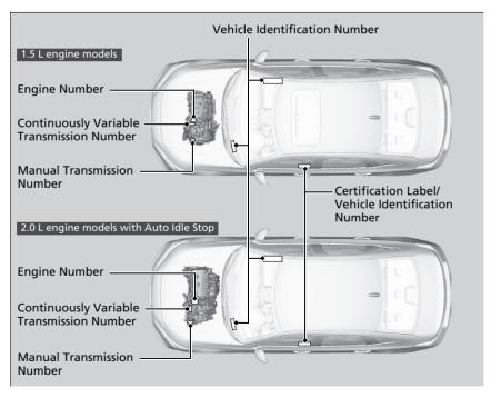
■ Vehicle Identification Number (VIN), Engine Number, and Transmission Number
