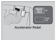
Depress the accelerator pedal while the transmission is in a position other than  $\boxed{\mathbf{P}}$  or  $\boxed{\mathbf{N}}$ . The system is canceled and the vehicle starts to move.
