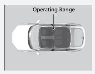
The engine may also start if the keyless remote is close to the door or window, even if it is outside the vehicle
