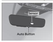
When you are driving after dark, the automatic dimming rearview mirror reduces the glare from headlights behind you. Press the AUTO button to turn this function on and off. When activated, the AUTO indicator comes on.
