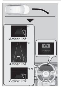
The front wide view camera behind the rearview mirror monitors left and right lane markings in white or yellow, the outer edge of the pavement (bordered by grass or gravel) or a detected oncoming vehicles.
