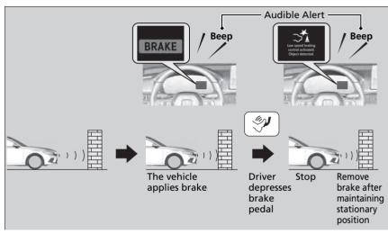
If the only rear sensors are turned off using the parking sensor system, the Low Speed Braking Control will not work when reversing.
