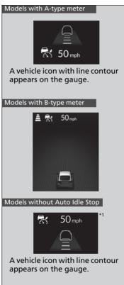
Your vehicle maintains the set speed without having to keep your foot on the brake or accelerator pedal.
