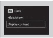
Roll the left selector wheel to scroll to select Display content, then press the left selector wheel.
