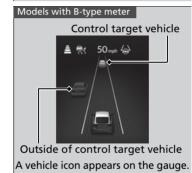
Control target vehicle: White and outlined in green Outside of control target vehicle: Gray
