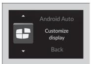
1. Roll the left selector wheel until **Customize display** is selected, then press the left selector wheel
