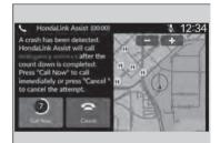
If your vehicle's airbags deploy or if the unit detects that the vehicle is severely impacted, your vehicle automatically will attempt to connect to the HondaLink operator. If connected, information about your vehicle, its location, and its condition can be sent to the operator\*1; you also can speak to the operator when connected.
