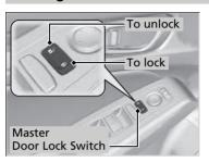
Press the master door lock switch in as shown to lock or unlock all doors, hatch and fuel fill door.
