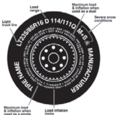
Figure 4: Typical Light Truck Tire Markings
